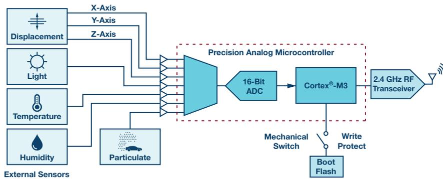
Figure 4. Physically write protecting firmware, except when performing an update, is an effective way to protect the integrity of a device.
